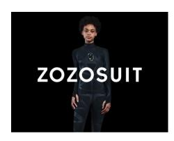
The "ZOZOSUIT" is a body measurement suit with built-in stretchable sensors, which was co-developed between Start Today and "StretchSense Limited", a soft stretch sensor development company in New Zealand.
